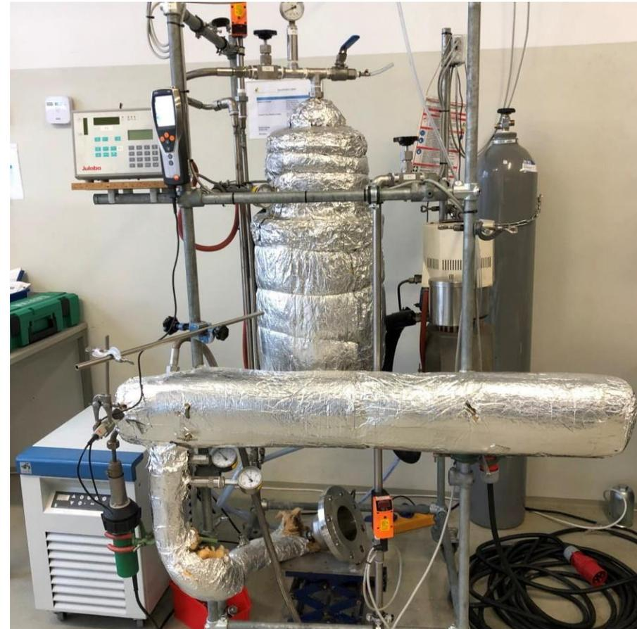
Pilot plant for CO<sub>2</sub> capture and storage in ttz Bremerhaven
